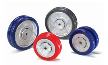
Choice of Four Durometers: 70A (Black), 80A (Red), 95A (Blue), 60D (Gray) Tread Types: CR: Crown or FT: Flat Tread Diameter Sizes: 3", 4", 5", 6", 8", 10" Axle Sizes: 1/2", 3/4", 1" and 1-1/4"
