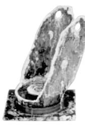
Dichromate Zinc Plating failed after 72 hours.
