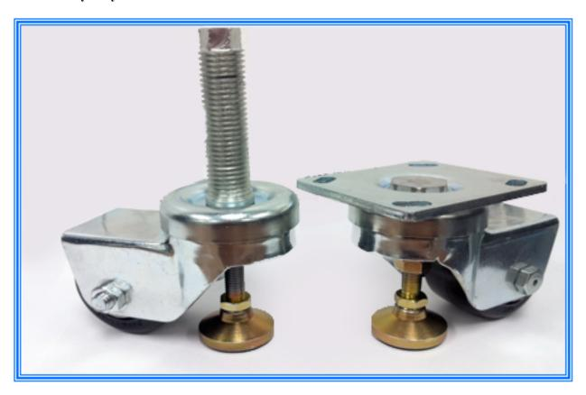
LevelMaster is designed and engineered so that each caster can easily handle a maximum load up to 1000 lbs. Available in either plate or stem mounted options, the LevelMaster also features a shock absorbing non-slip rubber leveling pad for improved stability when engaged with floor surfaces.
