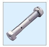
CROSS DRILLED AXLE Standard on 60 and 70 series casters. Axle is drilled through center. Allows grease to flow into the bearing. GREASE FITTING IN AXLE Standard on 400 series optional 60 and 70 series. Cross drilled axle with zerk fitting in end. Fits standard grease guns.
