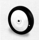
Same as JEX, however electric conductive Tread: rubber, black, non-staining, Shore A 75, with threadguards, precision ball bearing, sealed, temperature range from -20 to +85°C
