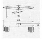
**Double lever** flat shape with rat-trap pedal.
