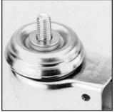
**S70 Threaded Screw** The screw is inserted loose into the housing. In the case of 2477 it is screwed in. 2471, 2477 & 2478 casters have to be secured against turning, when mounted to the equipment.
