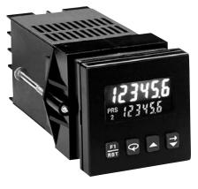
The 83 Counter features a 7 segment, 2 lines by 6-digit backlit LCD display. The main display line is red and shows the count value or the batch/ total value when preset 3 or output 3 is viewed in the secondary display. The smaller secondary display line is green and can be used to view the prescaler value, preset values, output count values or batch/total count values (batch model only).
