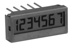
The Model 54 is a 7 or 8 digit LCD Totalizer with PCB mounting. Ideal for applications where PCB mounting, high reliability and long life are important. Units are 7 or 8 digits and come with their own lithium battery. Totalizers have two count speed ranges, 40cps or 150cps and are customer selectable.
