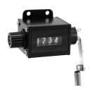
This 3 or 4 figure stroke counter with operating lever, spring assembly and reset knob, requires minimal space for mounting plus offers a high count rate and long life. The Model PCU can be reset during operation without damage. All PCU's are designed to minimize internal contamination, making them an excellent choice for outdoor use.
