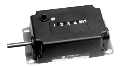
A 5 figure medium duty counter designed for applications where a rotary counter with a quick reset is desirable. When a 1' circumference measuring wheel is used with our standard counter, the counter will display feet and inches. Consult the factory if you have custom applications.
