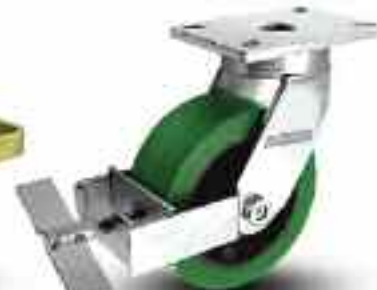
Face Contact Brake (FCB) Turn lever to apply shoe against wheel tread for positive locking action. (Recommended for Pneumatic casters.)
