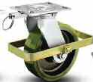
Wrap Around Brake (WAB) Foot operated on both sides. Use with straight roller bearing. Overall height must be greater than 5-1/4".
