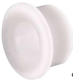
Delrin is a high-strength, wear resistant material with a low coefficient of friction. This combined with good chemical resistance and low moisture absorption make it ideal for use as a wheel bearing. This is our standard stainless bearing. One-piece Delrin bearings are required when a cam-style brake (BR) is used.
