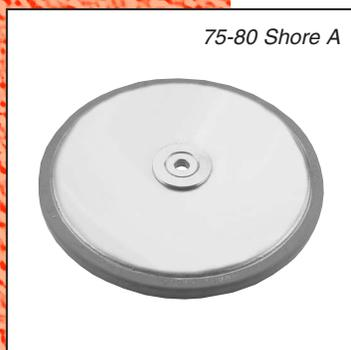
Designed to fit almost every type of portable equipment requiring heavy duty bumpers. These solid rubber bumpers with a heavy steel insert are made of grey non-marking rubber, molded around the steel insert making the entire unit virtually indestructible and long lasting. The machine steel hubs are made in the following sizes: 7/16", 1/2", 9/16", 5/8", 3/4", 13/16", 7/8" and 1". Other sizes available on request.
