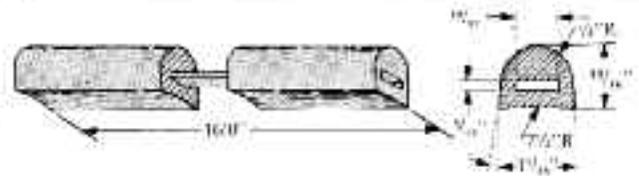
**MODEL A-567** is a flat-based rubber strip designed for installation on either metal or wood surfaces. This model is easily applied and does not require a special channel. Wt. 9 oz./ft. Metal insert optional.
